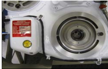
Figure 2. Cold Spray Repaired Hydraulic Pac Surface
