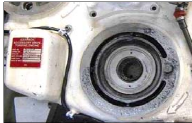
Figure 1. Fretting Damage on Hydraulic Pad Surface
